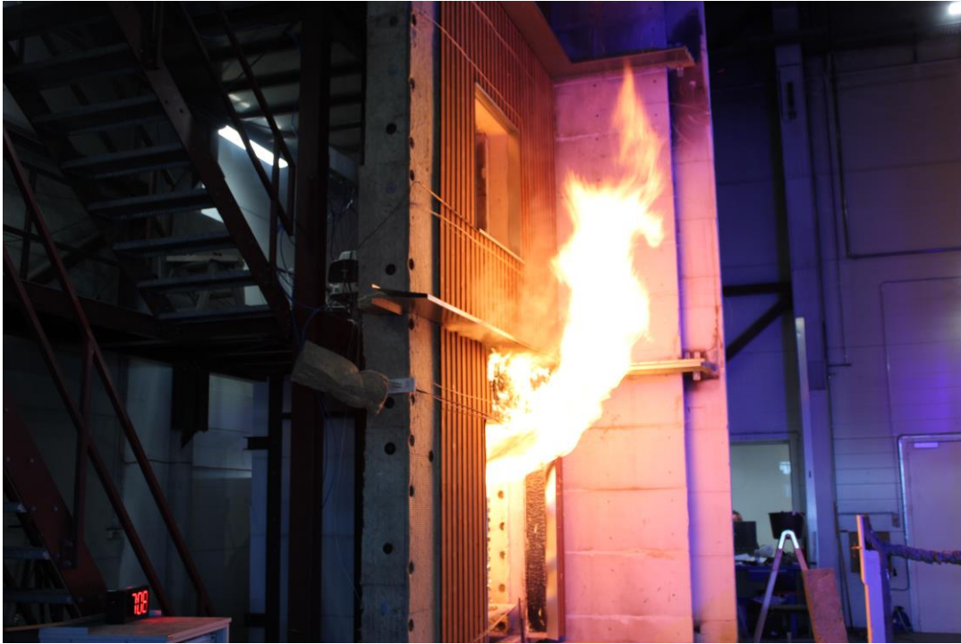
Photo No. 13 Test specimen 7 minutes into the test
