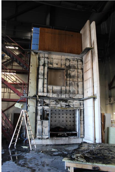
Photo No. 23 Test specimen after the test
