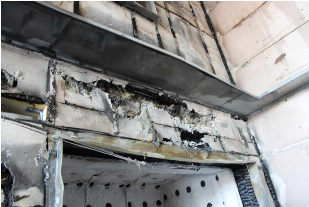
Photo No. 24 Test specimen after the test. Detailed photo below the first flame deflector
