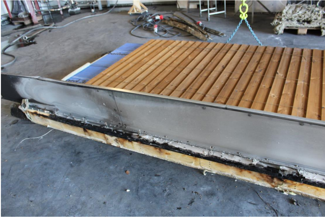
Photo No. 27 Test specimen after the test. Detailed photo of top prefabricated cassette
