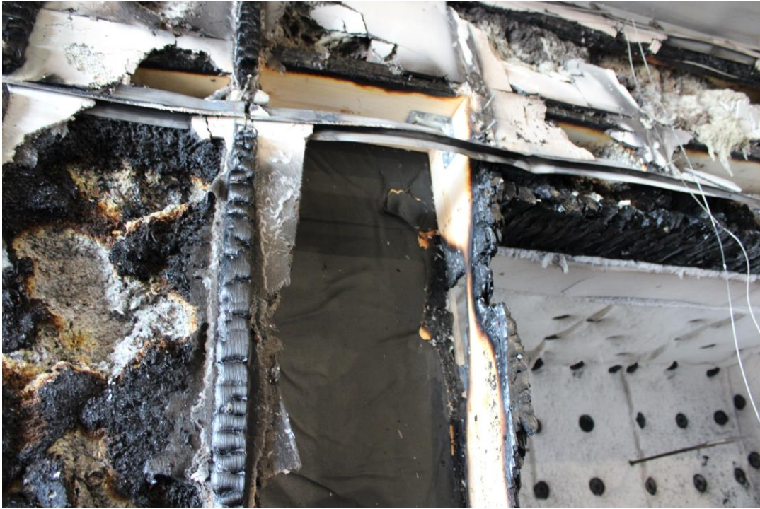
Photo No. 25 Test specimen after the test. Detailed photo of corner below the first flame deflector
